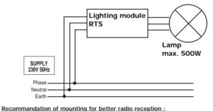
minimum distance between LIGHTING module RTS and the floor: 1,5 m.
