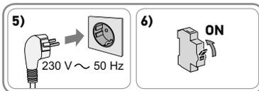
**h** The mains sockets must be installed close to each device component and must be easily accessible.
