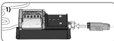
2) Connect the cable on the male Hirschmann plug side with the right or left Hirschmann female output of the EMS2 AC Power Box.
