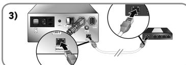
4) Connect a second RJ45 cable between the Ethernet ports of the Ethernet HUB and the EMS2 Touch Panel.
