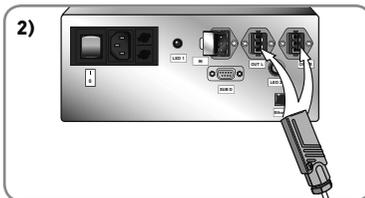
**i** Two outputs are provided to allow, if necessary, the connection of two EMS2 Connection Boxes, one for positioning to the left of the assembly table, the other for positioning to the right.
