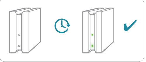
To improve the radio range, we recommend that the TaHoma® box be placed in an unconfined place in the middle of the house (avoid metallic surfaces and enclosures).
