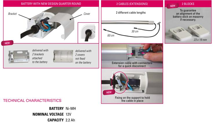
AMBIENT TEMPERATURE OF USE from -20°C to +70°C PROTECTION INDEX IP X4 LIFETIME ± 8 years DIMENSIONS & WEIGHT 570 x 27 x 27 mm with 0.3 m cable (2-point connector) - 730 gr 570 x 27 x 27 mm with 0.6 m cable (2-point connector) - 760 gr
