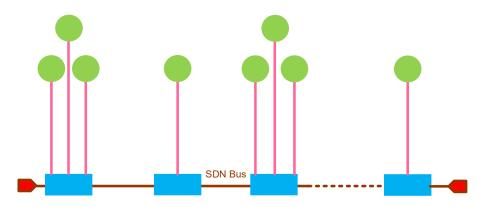
SDN bus: The maximum length cannot exceed 1200 m / 4000 ft and refers to the controller documentation. Junction: **passive** must be used.
