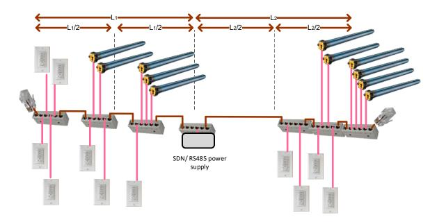
L1: the current needed by powered devices is 250mA. Chart-> max. possible 320 m
