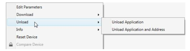
When the device has been programmed with the ETS software, a reset in the delivery state is no longer possible via the Rest/Prog button. Over the function "Unload" in the ETS, all settings of the device can be set back in the delivery state. The Reset/Prog button is then freed again.
